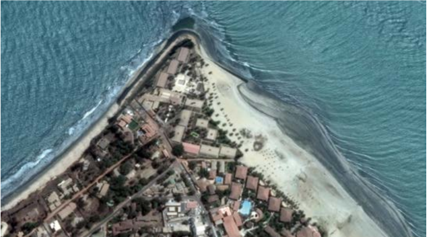
Developments at Cape point (armoring at the west of the Point, curved groynes filled in the East) (Source : Google Earth 2015).
