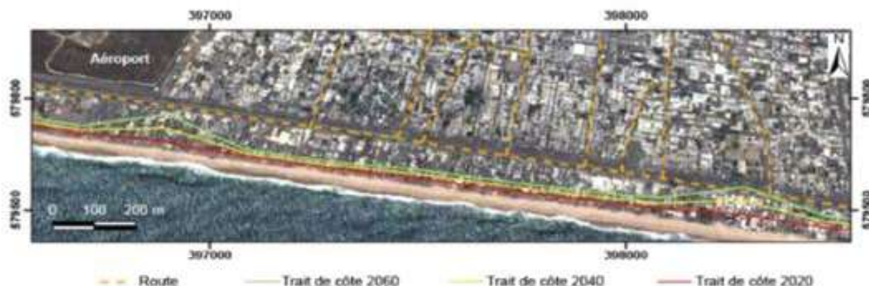
Future cut scene of the shoreline along the Airport-Anani highway (source Koffi et al., 2014)
