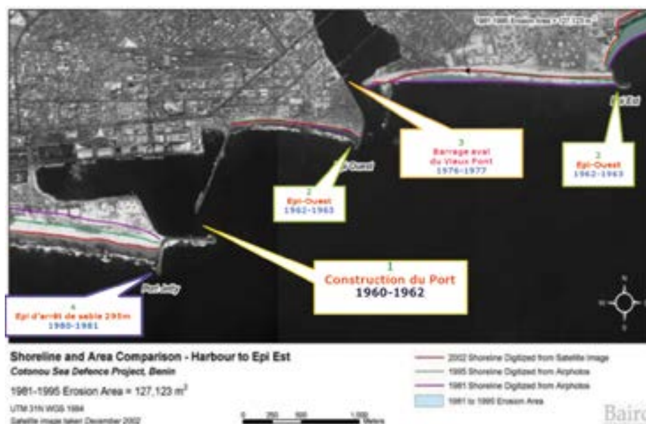
Distribution of protection works around the port (source: SDLAO, National Study, Benin)
