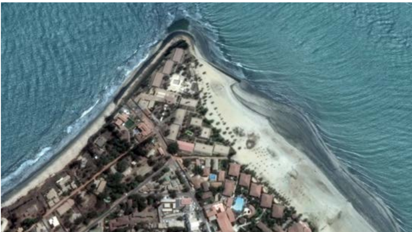
Developments at Cape point (armoring at the west of the Point, curved groynes filled in the East) (Source : Google Earth 2015).
