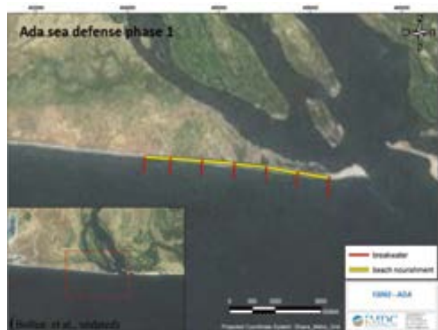
Shoreline protection project of Ada, stage 1 (source: MOLOA Ghana country branch)
