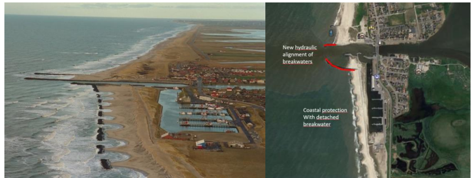
Figure 2.2: Example of design of breakwaters and downstream protection with detached breakwater. Left: Before adjusting breakwaters; Right: new alignment based on hydraulic modelling. Source: "Shoreline Management Guidelines" DHI 2017
