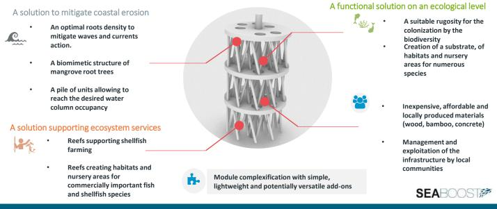
ROOT RELIES ON THE WORLD BEST PRACTICES TO UNDERSTAND AND MODEL DYNAMICS IN ORDER TO MITIGATE COASTAL EROSION. IT IS A POROUS MODULAR STRUCTURE, WHOSE SETTLEMENT PATTERN AND DIMENSIONS ARE CUSTOM-MADE AND ADAPTABLE TO BEST FIT AND EVOLVE WITH THE LOCAL CONTEXT.
