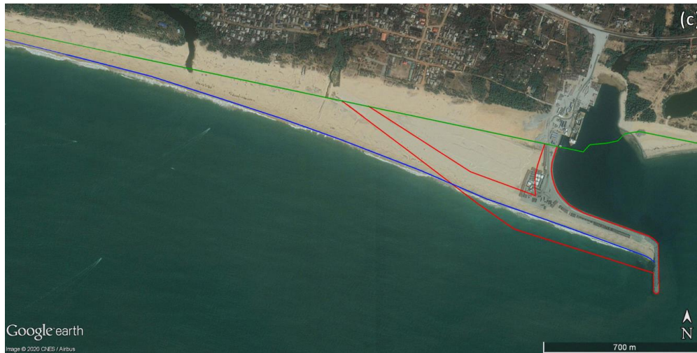
Figure IV.5 Satellite image from 24 December 2018 (Google Earth) with green line: showing the coastline just before construction sandbar body, red line: showing the situation just after the sandbar body has been put in place according to the design and blue line: showing the resulting reshaping after a wet season and the coastline reaching the equilibrium coastline orientation as expected
